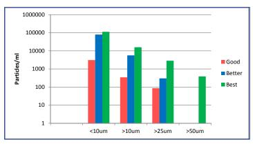
Figure 1: Differences in measured size distributions caused by variations in grayscale thresholding for the same sample.
