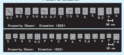
Typical volumetric-based particle analysis techniques, like laser diffraction and light obscuration, do not provide particle shape information - they assume all particles are a sphere. FlowCam Biologics can distinguish between protein aggregates and silicone droplets based upon particle shape, even in the 2µm to 10µm size range (due to superior image quality) as shown above.
