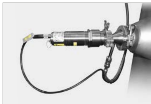
The pyrometer measures the highest temperatures up to 3000 °C. The pyrometer is focused to a specific location in the hot area. The heat radiation is transmitted through a quartz glass and measured by the pyrometer's sensor. An integrated gas tube ensures gas flow along the quartz window. The pyrometer can be adjusted by the sliding thermocouple.
