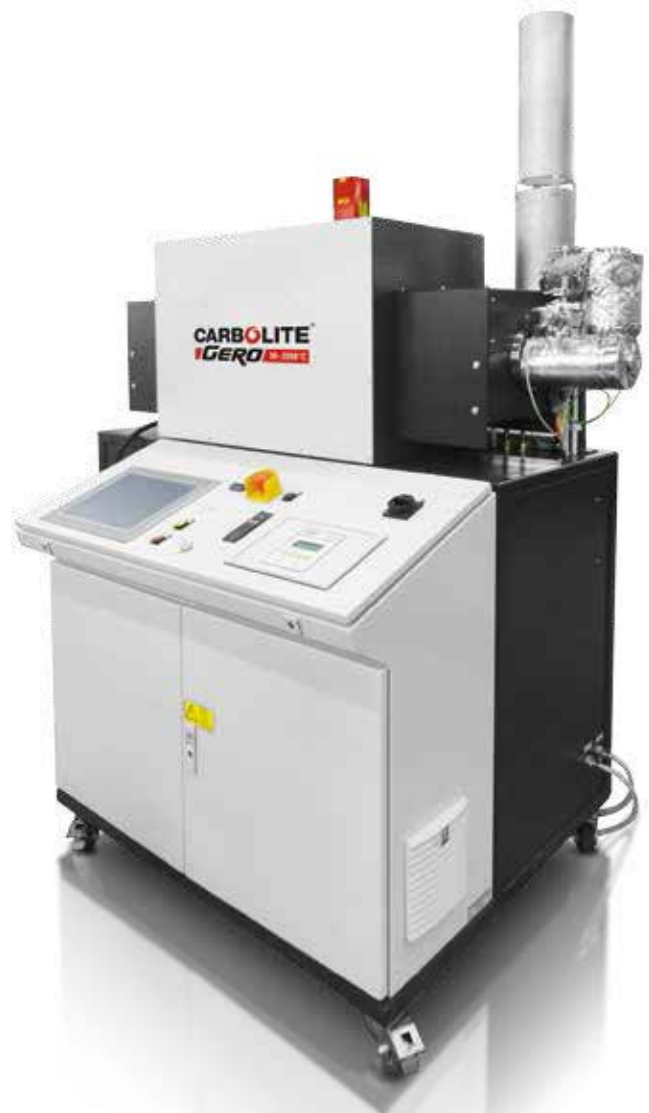
HTRH 16/100/600: Hydrogen tube furnace with a heated length of 600 mm up to 1600°C. Operation under pure Hydrogen is possible. All safety provisions are implemented.
