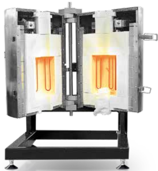
HTRV-A 17/70/250: High temperature vertical split tube furnace with a heated length of 250 mm up to 1700°C.
