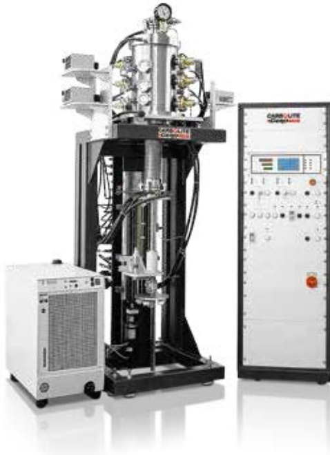
Special Bridgman growing device up to 2200°C: The samples is slowly pulled out of the hot area into an InGa bath. InGa is a liquid metal with a low vapor pressure. With this system, the highest possible temperature gradients are possible.
