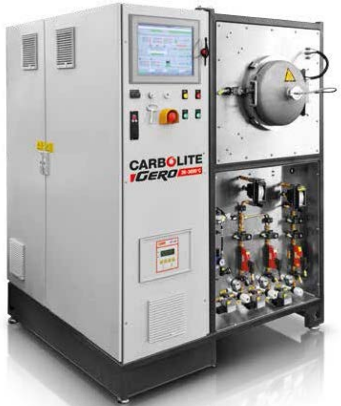
GLO 40/11: Annealing furnace with a usable volume of 40 l up to 1100°C under atmospheric pressure.
