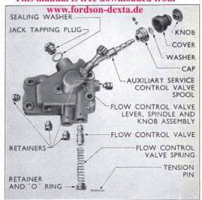
Fig. 58 **Auxiliary Service Control Plate and Flow Control Valve**
