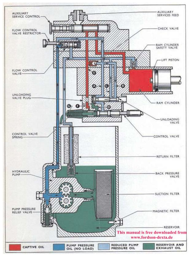
Fig. 55 **Hydraulic Oil Flow - Neutral**
