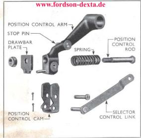
Fig. 31 **Position Control Linkage Assembly**
