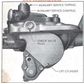
Fig. 2 Lift Cylinder and Auxiliary Service Control
