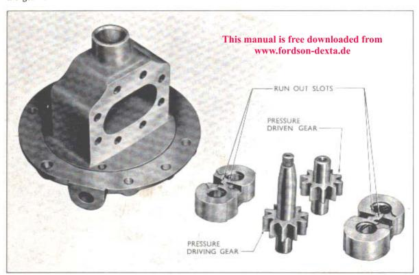
Fig. 42 **Hydraulic Pump Body, Bearings and Gears**
