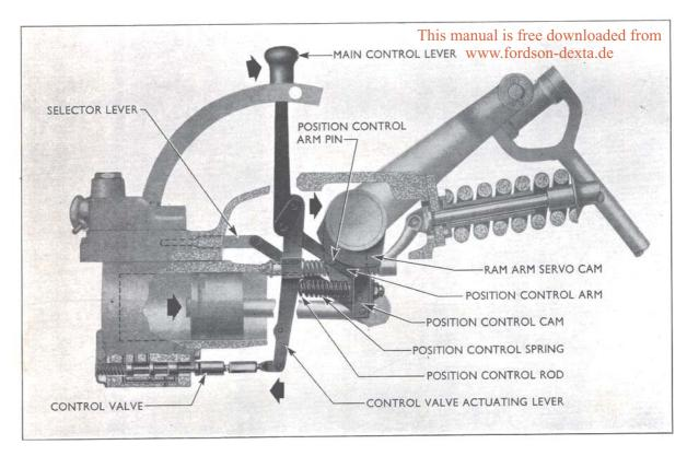
Fig. 9 **Position Control Linkage - Raising**
