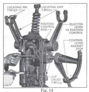
Position Control Linkage Adjustment
