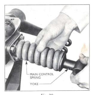
Fig. 38 **Main Control Spring Adjustment**
