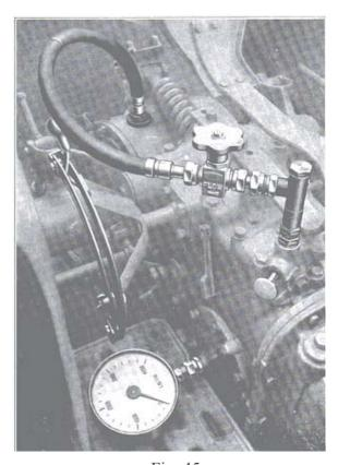
Fig. 45 **Hydraulic Pump Test Equipment**
