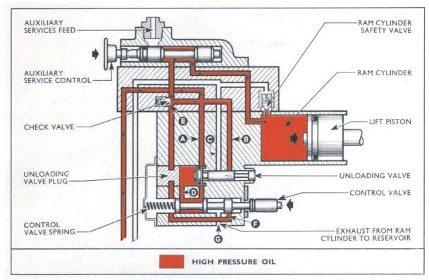
Fig. 11 **Hydraulic Oil Flow - Raising**
