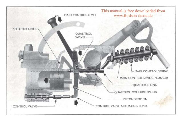
Fig. 6 **Qualitrol Linkage - Lowering**
