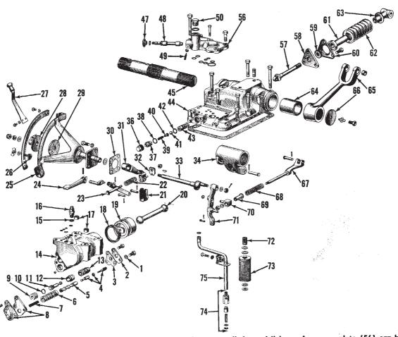
Fig. FO563 — Exploded view of early Fordson Dexta hydraulic lift cover, cylinder and linkage. Accessory plate (56) can be replaced with flow control valve (54—Fig. FO564) if complete valve and linkage are used. Although component parts are different, complete lift cylinder assembly (14) is interchangeable with later type complete lift cylinder assembly (14A — Fig. FO564). - Fig. FO564).
