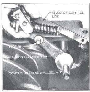
Fig. 32 Assembly of Position Control Linkage to Cover
