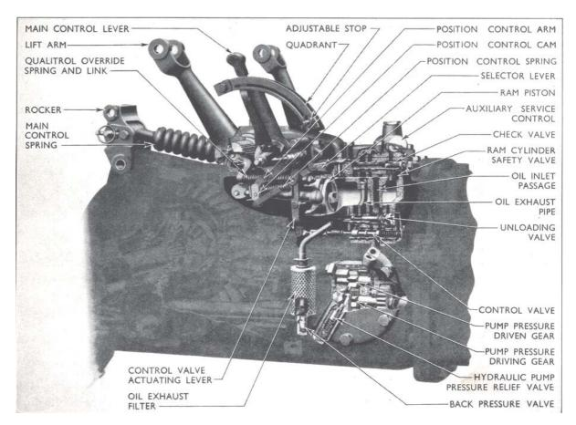
Fig. 1 Sectioned View of Hydraulic System
