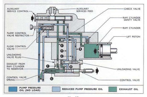
Fig. 57 **Hydraulic Oil Flow - Lowering**
