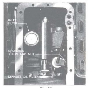
Fig. 39 **Location of Exhaust Oil Filter Assembly**
