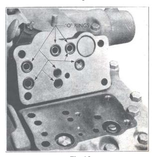
Fig. 15 **Auxiliary Service Control Plate**
