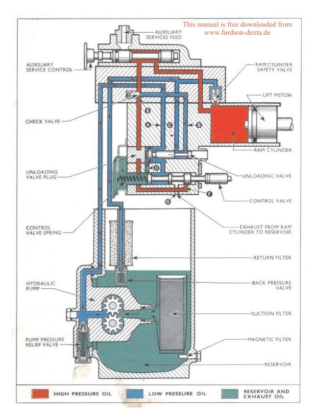
Fig. 10 **Hydraulic Oil Flow - Neutral**
