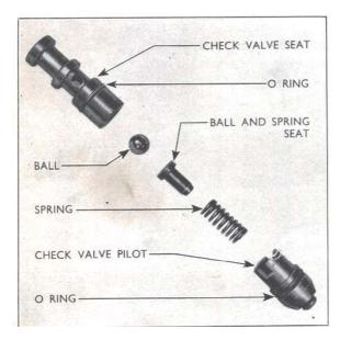
Fig. 16 Check Valve Assembly
