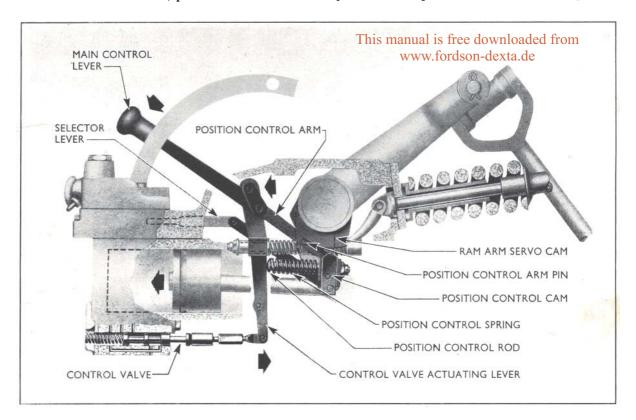
Fig. 8 **Position Control Linkage - Lowering**
