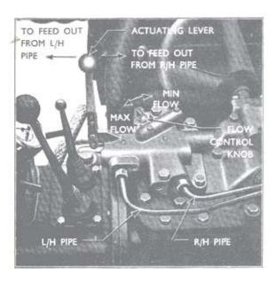
Fig. 47 **Actuating Lever and Flow Control Knob**
