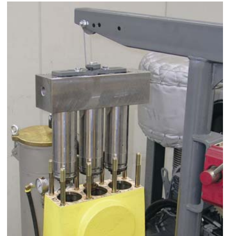
Step 3: Lift out the complete medium bearing end and store. Fit the new medium bearing end in the reverse order.
