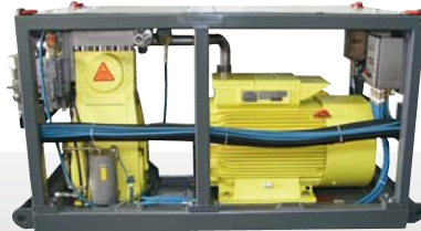
Transportable unit with extra strength base and frame for deep mining applications
