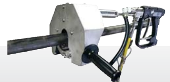
Hand rail cleaner removes rust and old coatings down to bare metal prior to recoating
