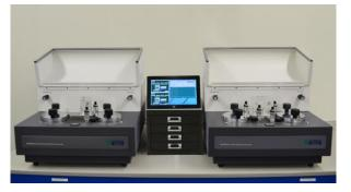
Systech have been designing and manufacturing oxygen permeation and water vapour permeation analysers for many years offering reliable and versatile testing of all films, packages and bottles. With precise control, these analysers offer a wide sample temperature range of 5° to 50°C and a measured and controlled relative humidity range of 20 to 90% RH. All Systech analysers are certified traceable to NIST.
