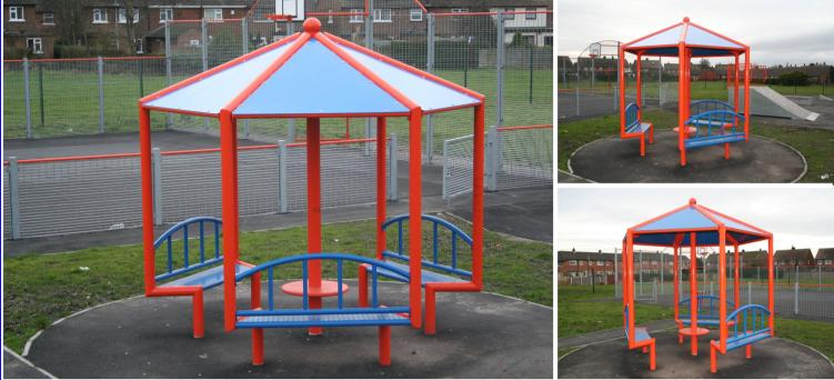
Assembled using stainless steel tamper resistant bolts, they can be concreted into place, or bolted down onto a galvanised steel floor, this is simply fixed to any level surface by means of a ground anchor system, enabling the shelter to be removed and re-sited if necessary. With gloss powder coated roofs and no hand or footholds they are designed to deter climbing.
