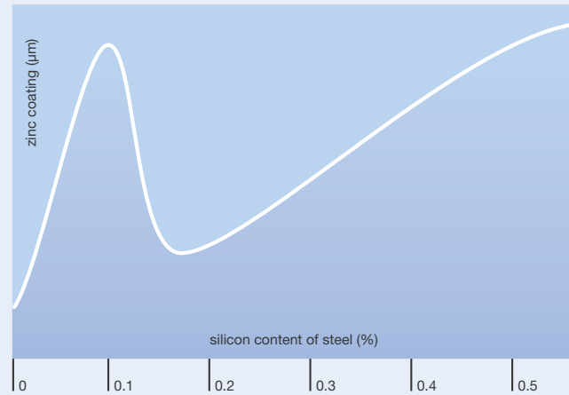
Fig. 5. Approximate thickness of the zinc coating to the silicon (Si) content of the steel. (This is a schematic representation, please contact Galvanizers Association for detailed information)
