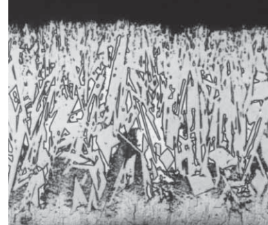
Fig. 4. Microstructure of the thick coating obtained using a silicon-rich steel.
