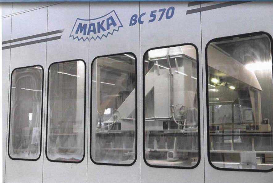
▲ capricorn uses Maka's 5-axis CNC technology for component trimming and model making purposes
