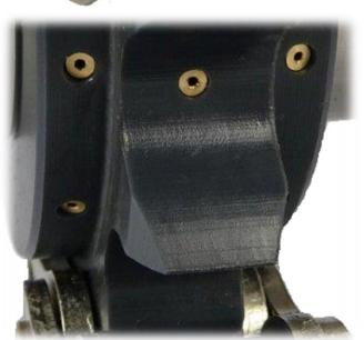
Rotalube was introduced on a chocolate production line, replacing a traditional brush lubrication system. Because Rotalube applies an accurate, controlled amount of lubricant - and, unlike the brush system, doesn't over lubricate - the customer benefitted from less down time, as they no longer had to regularly stop to clean the contaminated chain and sprockets.
