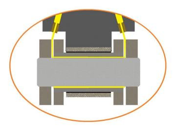
No matter what the chain speed, or its elongation, Rotalube very precisely applies an accurate amount of lubricant to the target pins and bushes.
