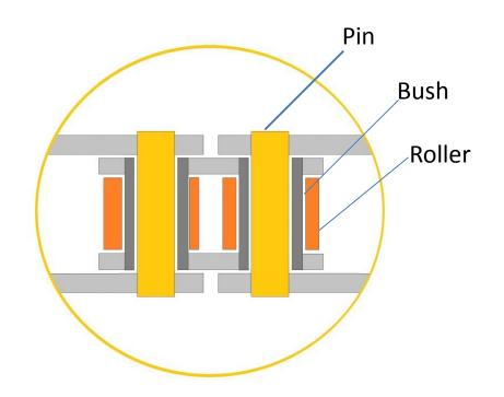
A roller chain is a series of connected journal bearings that articulate as they enter and leave the sprockets driving them. This articulation results in wear on the pins and bushes. As material is worn away from these surfaces, the roller chain gradually elongates
