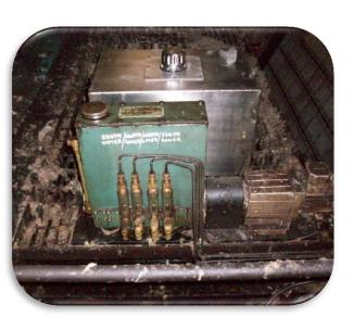
Rotalube replaced oil spit/spray system on Forming oven saving \$80K Per year in oil.
