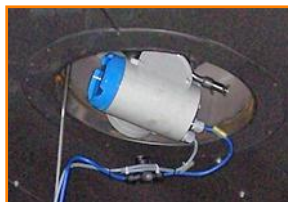
Sonatec HW with sample point & CIP nozzle
