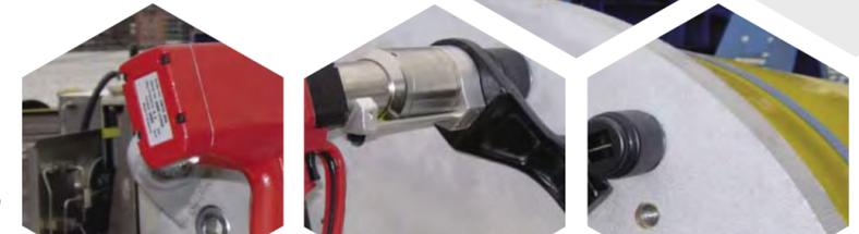
Pneutorque fitted with torque transducer and angle encoder, shown with torque and angle or turns measuring instrument.
