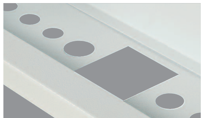
Wide range of Circular Conduit holes and square cut out for trunking, these are all laser pre cut so as to give easy access without damaging the Gland Plates.
