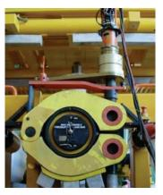
Norbar have developed a torque multiplier specifically for actuating wet pipe connector clamps requiring torques up to 63,000 N.m. The tool is mainly constructed of high strength aluminium to keep the weight within the limits of a standard ROV.
