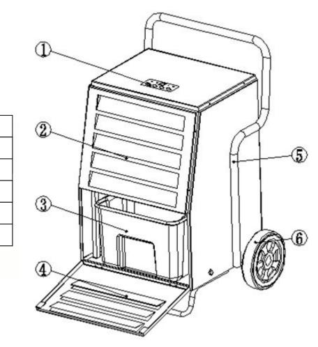
Control panel Filter grid Water tank Tank cover Handle
