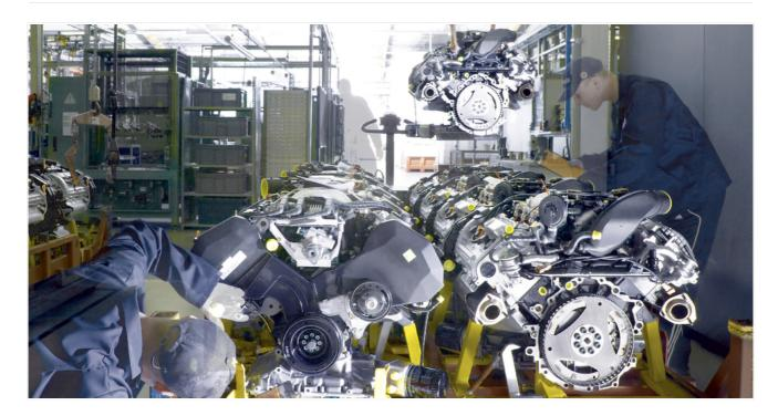
Sub-assemblies are an integral apart of a manufacturing process. MAHLE Powertrain incorporates these processes into it own Powertrain assembly lines to allow uninterrupted and balance flow of the main assembly line. Typical assemblies are cylinder heads, inlet systems, turbo charging systems, pistons and oil pans.
