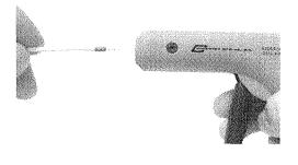
Remove the crimped wire with ferrule.
