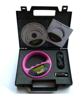
The scanner is designed to read all ISO FDXB chips. It generates a small magnetic field that activates the microchip when within range. The chip will respond if within about 4" and the scanner will display the microchip's unique ID number on its LCD screen with an audible 2 beeps.
