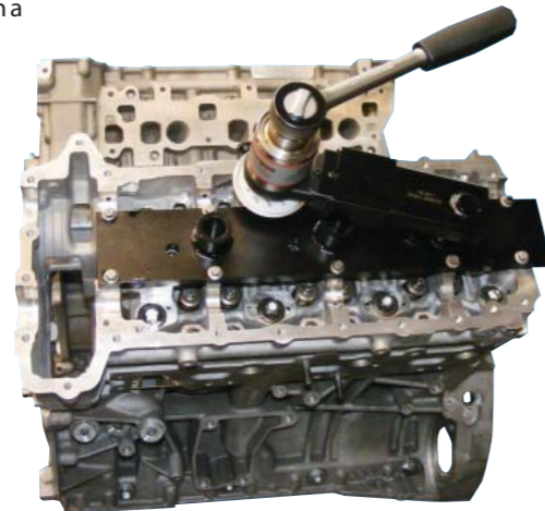
Hand torque multiplier fitted with torque bar adaptor, special torque reaction arm and angle gauge assembly
