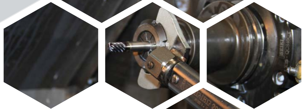
Special fitting for torque tightening of tool collets. Undertightening can result in the collet not holding the tool whereas over tightening can cause damage to the collet.
