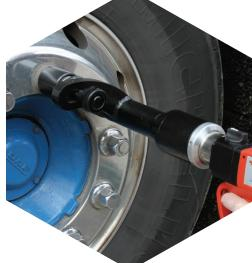
TruckTorque™ incorporating the sliding 'banana' reaction
