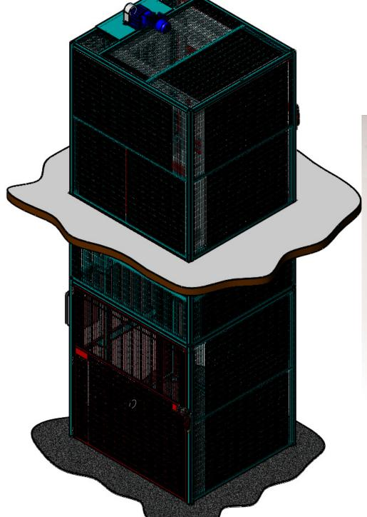
**Description:** Goods only mezzanine floor lift, with no operator access to platform for loading/unloading
