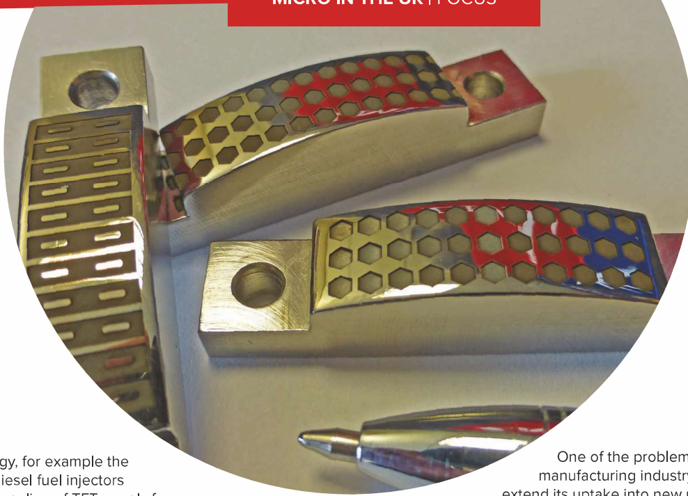
<< Figure 4: Laser micro machined curved mould tool inserts. >>
