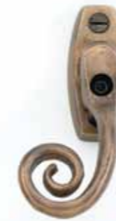
470 Espag. Fastener (lockable) 42mm screw centres, 7mm spindle (handed – left hand shown)
