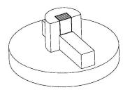
**Figure 3:** Illustration of the cutting assembly used for mounting and cutting the specimen stacks into a long rod. The specimen rod is then mounted into a brass tube used as the support ring and to provide mechanical support to the stack when thin.
