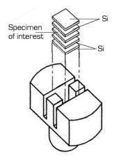
Figure 2: Illustration of the use of the bonding jig for constructing the specimen stack for cross section specimen preparation. The sacrificial stacks of Si are placed both on top and below the actual specimen of interest. In between each square piece of material is where the epoxy is applied. The entire jig is then placed into the specimen clamp to create a thin layer of epoxy in the specimen.
