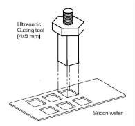
**Figure 1:** Illustration of the cutting tool used on the Model 380 for the production of the stacking materials for preparing stacked specimens. These  $4 \times 5$  mm Si pieces will then be used as the bonding material for making the actual specimen thicker. Cutting times for each individual square was ~ 45 seconds.
