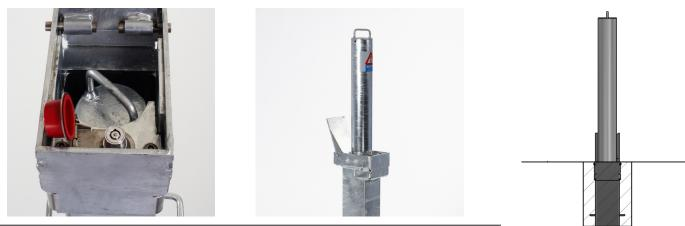
The RetractaPost-GL offers a highly effective and robust way to protect premises and vehicles. The RetractaPost-GL is raised and lowered vertically. When raised the post is 500mm above ground, when lowered the post is fully below ground and covered using the integral lid. The post is lockable in the raised position by rotating the post 45° and then pressing the high-security push button 7-pin security lock. The post is unlocked using the supplied key, rotated and then lowered.
