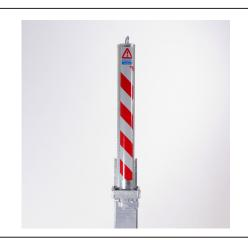
The RetractaPost-GL offers a highly effective and robust way to protect premises and vehicles. The RetractaPost-GL is raised and lowered vertically. When raised the post is 745mm above ground, when lowered the post is fully below ground and covered using the integral lid. The post is lockable in the raised position by rotating the post 45° and then pressing the high-security push button 7-pin security lock. The post is unlocked using the supplied key, rotated and then lowered.
