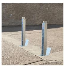
The Square RetractaPost-GL 900 is an effective means of preventing unauthorised vehicle access. When not in use, the post retracts into its integrated socket and is covered by the integral lid. The post is lockable in the raised position by rotating the post 45° and then pressing the high-security push button 7-pin security lock. The post is unlocked using the supplied key, rotated and then lowered.
