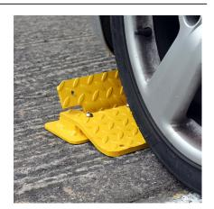
The AUTOPA Surface Mounted Flow Plates control traffic flow to one direction and are designed to work in groups to ensure full lane coverage. As a vehicles passes over the plate, the flap is pushed over allowing the vehicle to pass. Once the vehicle has passed the flap returns to its upright position.
