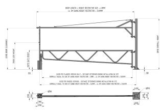
The AUTOPA Swing Height Restrictor with Swing Gate has a standard clearance of 2.05m, limiting access to high sided vehicles and is perfect for controlling access at retail park entrances. Whilst providing an effective barrier to vehicles of all sizes it can be opened as required to allow access to any vehicle.
