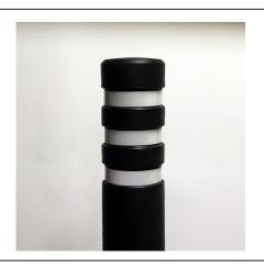
With a unique, slimline design, the EB300 bollard from AUTOPA is ideal for marking paths where space is at a premium. The EB300 bollard is highly versatile and features a galvanised steel core covered by a hard wearing medium density polyethylene (MDPE) sleeve. When complete with the core, this bollard can be installed at either 1000mm or 1200mm height above ground.
