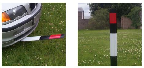
The Fleximarker Verge Marker is highly durable and suited to a wide range of roadside locations. Manufactured from UV resistant plastic, this verge marker complies with BS EN 1276-7. The Fleximarker flexes up to 90 degrees, returning to its upright position, and will not splinter in the event of an impact.
