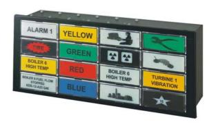
configured as group alarm, horn output and watchdog with a change over contact at the terminals. The group alarm can be set to one of four functions, Follows input, follows alarm, Multiple reflash, Ringback horn.
