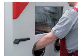
Manual access openings
