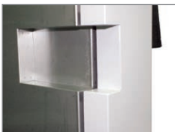
Notch-type access port in door
