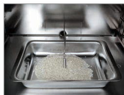
Specimen temperature display with PT 100 sensor
