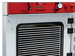
Vacuum drying oven with special racks for large numbers of particularly flat samples
