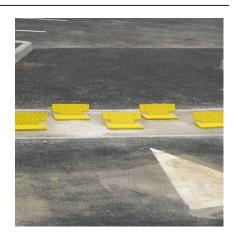
The AUTOPA One Way Flow Plate controls traffic flow to one direction only and is designed to work in groups to provide full road width coverage. As a vehicle passes over the plate, the flap is pushed down, allowing the vehicle to pass, the rubber buffer on the reverse of the flap ensures noise is kept to a minimum. Once the vehicle has passed the flap returns to its upright position.
