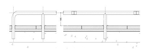
Designed with the retail market in mind, the AUTOPA Shop Front Protection Rail is ideal for protecting vulnerable walls and windows from trolley damage. Sitting only 185mm above the ground, this railing can be used to protect both internal and external structures and is commonly found around entrances or glass panels.
