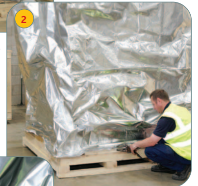
The bag is sealed to the base sheet.
