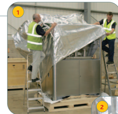
The base sheet is laid on the case base. Desiccant is added and the 3D bag is placed over the machine.
