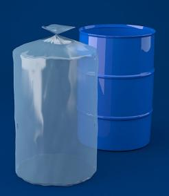
NITTEL Round Bottom Liners are manufactured by welding a circular disc to one end of an open ended tube of material. The weld then forms a liquid tight seal. This technology provides a high level of tear resistance. The accurate fit of the liner reduces the formation of creases and air pockets, which is often a problem with ordinary flat bags.
