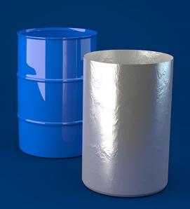
NITTEL Barrier Foil Round Bottom Liners are manufactured by welding a circular disc to one end of an open ended tube of material. The weld then forms a liquid tight seal. This technology provides a high level of tear resistance. The accurate fit of the liner reduces the formation of creases and air pockets, which is often a problem with ordinary flat bags.
