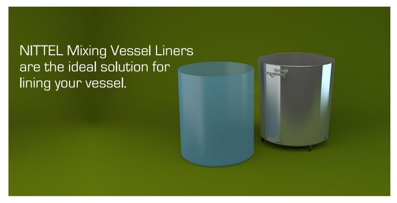
NITTEL Mixing Vessel Liners are manufactured by welding a circular disc to one end of an open ended tube of material. The weld then forms a liquid tight seal. This technology provides a high level of tear resistance. The accurate fit of the liner reduces the formation of creases and air pockets, which is often a problem with ordinary flat bags. Special discharge outlets can be fitted to the liner where appropriate.
