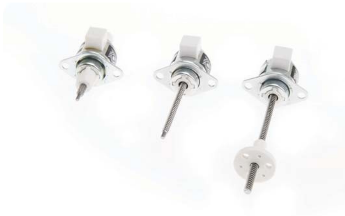
Figure 12. Can-Stack Linear Actuators. 19000 Series (20 mm) Captive, Non-captive and External Linear, available in 15 and 7.5 rotational degrees per step.
