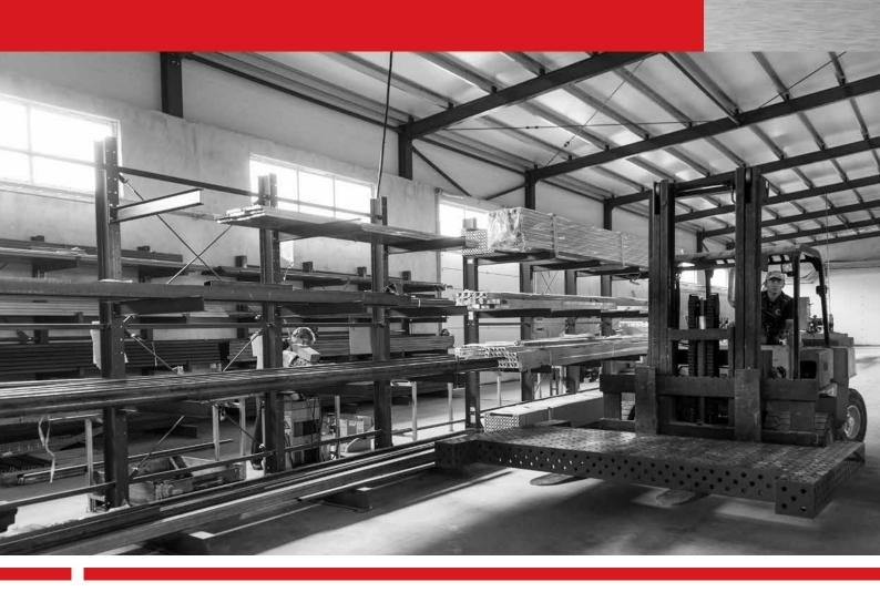
"Whether its plastic pipes, wooden planks or metal rods - cantilever provides an ideal storage method for long goods"
