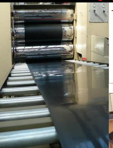
The granules are put through one of our extruders and made into new sheets ready for the vacuum forming machines
