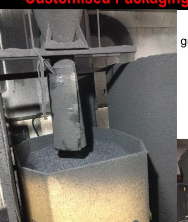
The pieces of plastic are put through one of our granulation machines and made into granules ready to be re-extruded into new sheet
