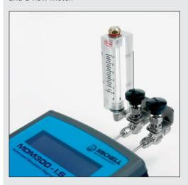
The Compressed Air Kit has a similar configuration to the Easi-fit Kit, but with the addition of a particulate filter and RP ¼" fitting, commonly found in the compressed air industry. The fitting is connected to the filter inlet by a 2m length of PTFE tube, to allow for flexibility when coupling directly to compressed air systems.
