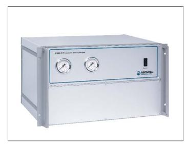
The Michell PSD Series Pressure Swing Dryers use two columns filled with 4Å molecular sieve desiccant, which are used alternately on a two-minute switching cycle. The PSD dryers are designed to operate continuously, using a small proportion of the dried air, to regenerate the offline column - generally giving desiccant life in excess of five years. This type of heatless regeneration also uses significantly less energy than a 'heated' type of dryer.
