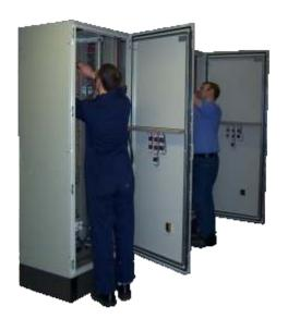
All control panels, incorporating PLC logic sequence and motor starters are designed and built inhouse to our demanding standards ensuring high reliability and compliance with current Health & Safety requirements.
