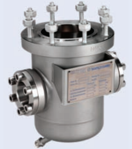
Type 4 Metal vessel with heating jacket, 2 sight glasses and drain valve 1.0 / 1.5 / 2.0 / 3.0 / 5.0 l max. 60 bar / 250°C
