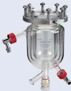
Type 1BI Glass vessel with heating jacket, drain valve and vacuum insulation jacket 0.5 / 1.0 / 1.6 l max. 6 bar / 200°C
