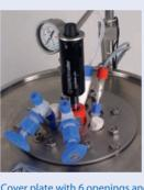
Cover plate with 6 openings and accessories made of PTFE, PFA, PEEK or glass
