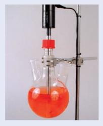
Installation of cyclone «i» with NS29/32 on round flask
