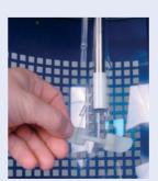
Installation of stirrer on glass tube Integrated motor with speed of magnetic drive cyclone «i»
