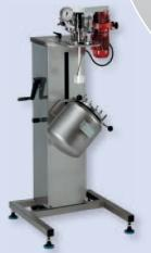
kiloclave with bmd 250 «i» and ATEX drive Glass lined steel vessels 1.0 – 20 liter Pressure max. 12 bar, max. 200°C Components and internals made of PTFE, PFA, glass lined or Tantalum
