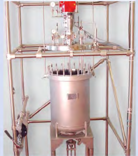
100 liter 50 bar hydrogenation reactor
