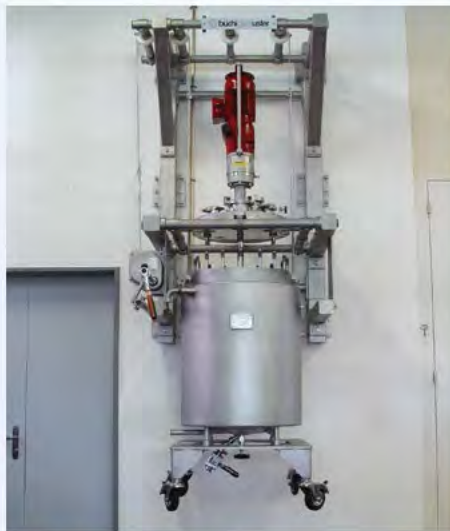
100 liter, 60 bar hydrogenation reactor, Hastelloy, cGMP, wall mounted
