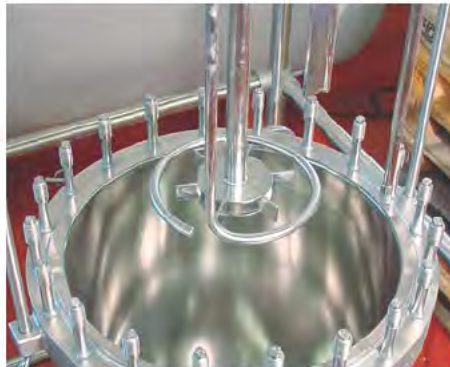
Turbine stirrer with gas inlet sparging tube for hydrogen
