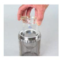
Vessel holder with protective wire mesh
