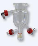
Type 1B Glass vessel with heating jacket and bottom valve 100/200/250/300 ml, 6 bar, 200° C
